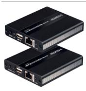
BCS-UTP-HDMI-SET converter set for HDMI signal transmission via UTP cable, transmitter + receiver, supports the solution "Point to point" and "point to multi-point"
